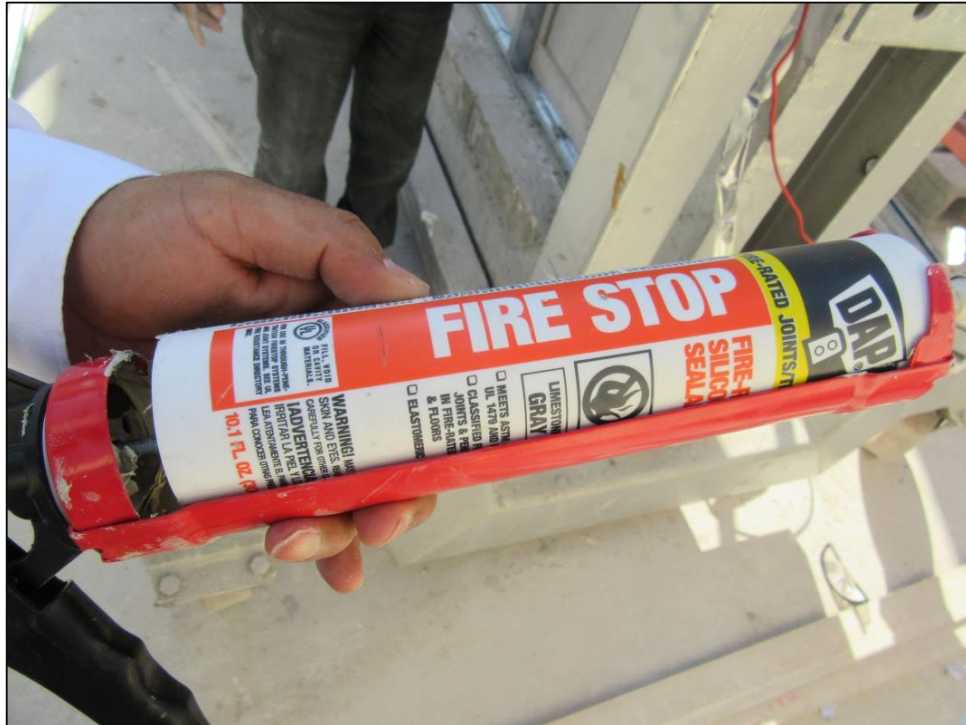
Picture 3: A photo of the sealant that was used around the perimeter of the framing system on the exposed face of the specimen.
