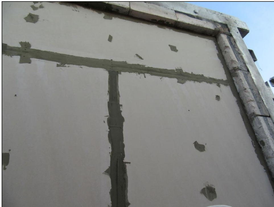
Picture 6: A photo of the cement jointing compound being used on the meeting edges of the boards, and the jointing compound being used alone on the screw heads and specimen perimeter.
